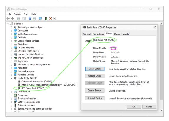
The above example shows a cable with an FTDI chip. A cable with a CH340 chip will display a manufacturer of "wch.cn". A cable with a SiLabs chip will display a manufacturer of "Silicon Laboratories". If you have a cable with a Prolific chip. you may see a message such as "PL2303x PHASED OUT SINCE 2012." or "PL2303x DO NOT SUPPORT WINDOWS 11 OR LATER". Ideally, you could return that cable for a
